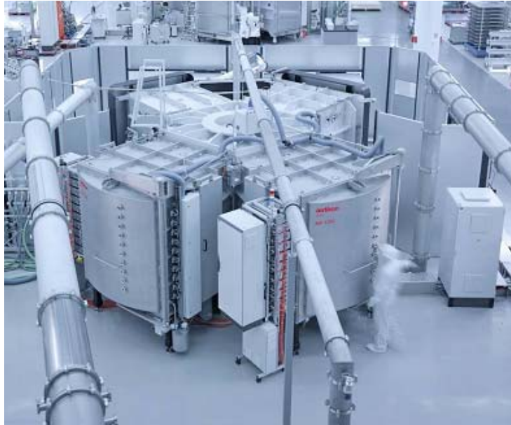
薄膜太阳能生产的核心：a-Si/ c-Si 镀膜设备 PECVD (Plasma Enhanced Chemical Vapor Deposition)
